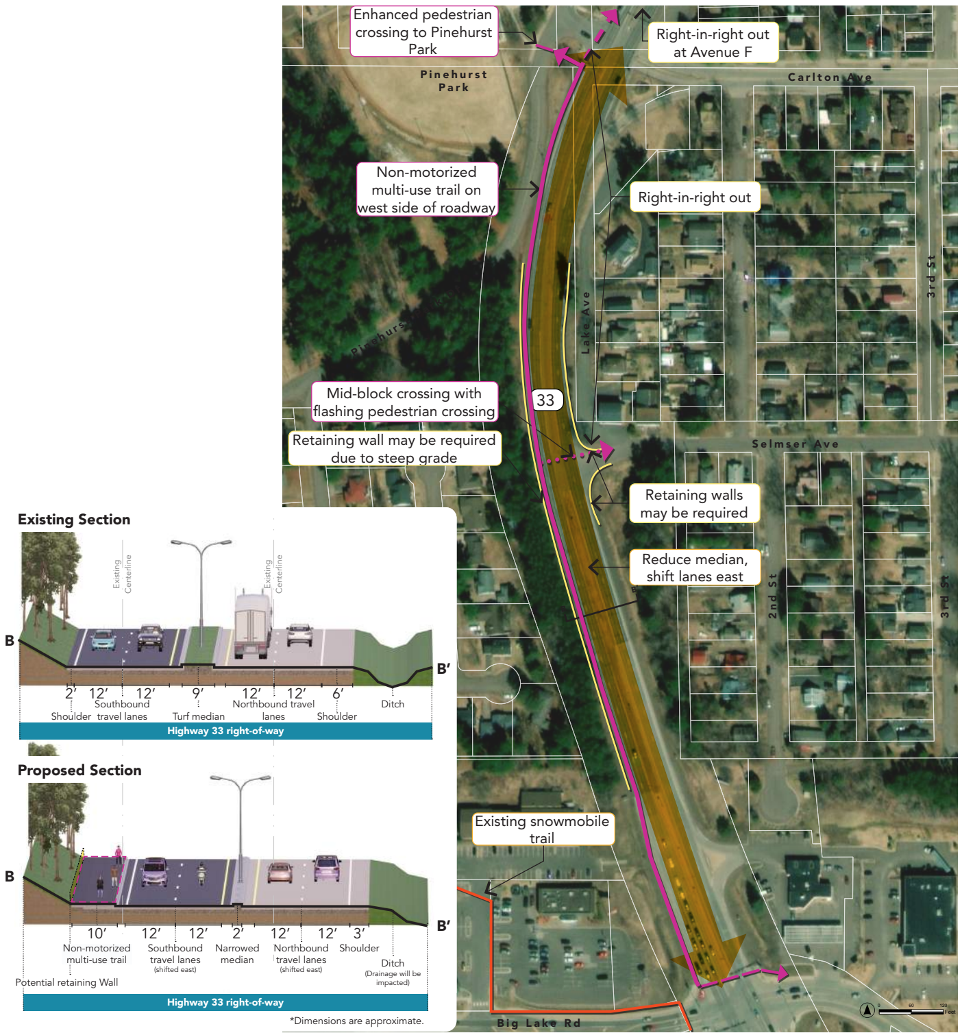
Figure 2 | Section 'B' Improvements
