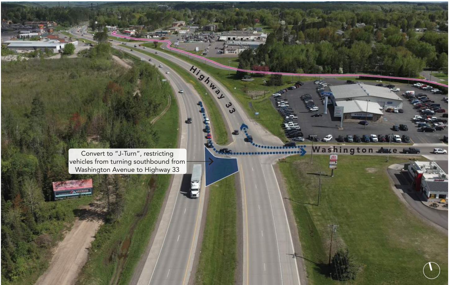
Figure 25 | Intersection Recommendations at Washington Avenue
